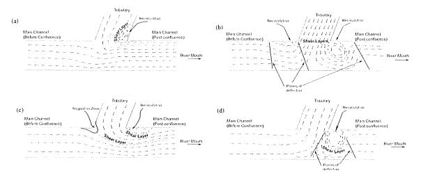
**Figure 7.** Schematic flow patterns of tidal confluence: (**a**) the maximum flood; (**b**) flood to ebb transition; (**c**) the maximum ebb; and (**d**) ebb to flood transition.
