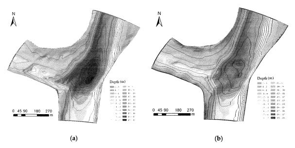
Figure 8. Measured bathymetry of a tidal confluence: (a) 2010; (b) 2015 (adapted from Xie [80]).
