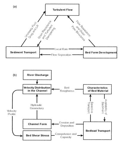
**Figure 3.** The conceptual relationship between flow, sediment, and morphology at a confluence, as proposed by (a) Leeder [11] and (b) Ashworth and Ferguson [12].
