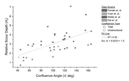
**Figure 9.** Relationship between  $H_r$  and  $\theta$ . The data source is from studies carried out by Ferrarin et al. [21], Yuan et al. [6], Wallis et al. [61], and Dai et al. [28].
