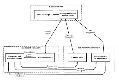
Figure 4. Unification of conceptual models by Leeder [11] and Ashworth and Ferguson [12].
