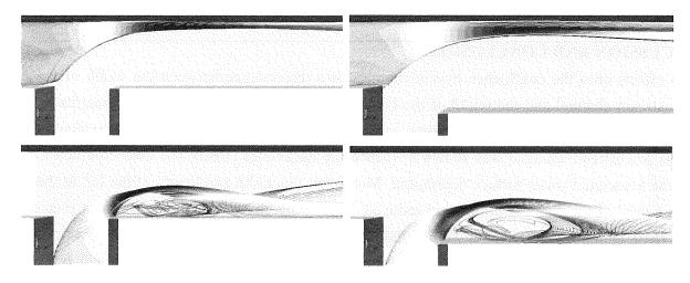
Figure 6. Streamlines of mean flow. Left panels: concordant width case ( $\omega$ =0.75), right panels: discordant width case ( $\omega$ =0.75). Top panels: streamlines originating from upstream main channel at an elevation of z/h<sub>d</sub>=0.12. Bottom panels: streamlines originating from tributary channel at an elevation of z/h<sub>d</sub>=0.12.
