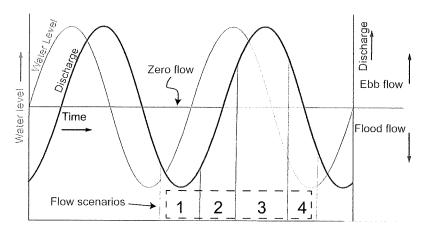
Figure 6. Schematic of flow scenarios used for studying the hydrodynamics of tidal confluences.
