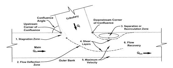
Figure 5. Six identifiable flow zones at a confluence—adapted from Best [32].
