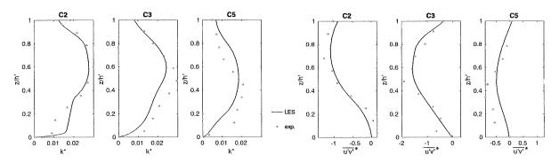
Figure 4. a. (left) Vertical profiles of dimensionless TKE ( $k^*=TKE/U_d^2$ ) in the core of the mixing layer in the discordant width case ( $\omega=0.75$ ); b. (right) Vertical profiles of the dimensionless (with respect to 10<sup>6</sup> x U<sub>d</sub><sup>2</sup>) Reynolds shear stress ( $\overline{u'v'}$ ) in the core of the mixing layer in the discordant width case ( $\omega=0.75$ ).
